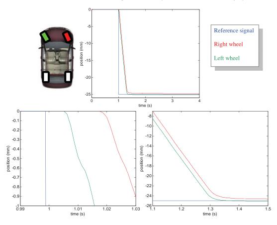
*Fig. 6. The directional control action member extension pattern – the left wheel as a Master, the right one follows it as a slave*
